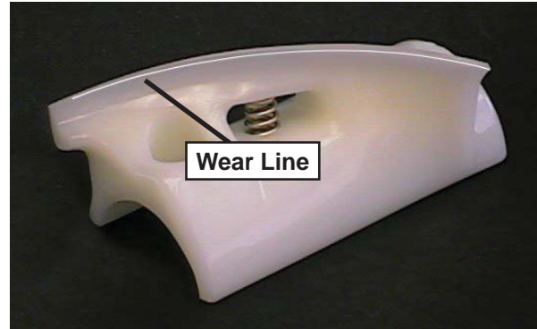
Figure 3-3 Auger Flight Wear
